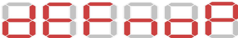
For the assignment, you are required to work out 7 minimal functions to calculate each of the seven segments, A to G, for the 16 possible input combinations. Show the 7 corresponding Karnaugh maps, and express the functions as a formula and network. Trace your network by the binary input for one of letters of your choice.
