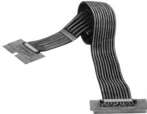
**Figure: The Unibus of the PDP-11 Computer**
